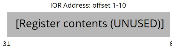
4. `ioctl(control_fd, CONTROL_TRIGGER_DENSE_ADDR, &vla)`: Finally, after hardware inputs the 10 dense results in their corresponding registers (done 1 clock cycle after receiving the previous `ioread32()` call), software does another `ioread32()` sweep across registers at offsets 1-10 to grab the CNN results and print them out to the user
