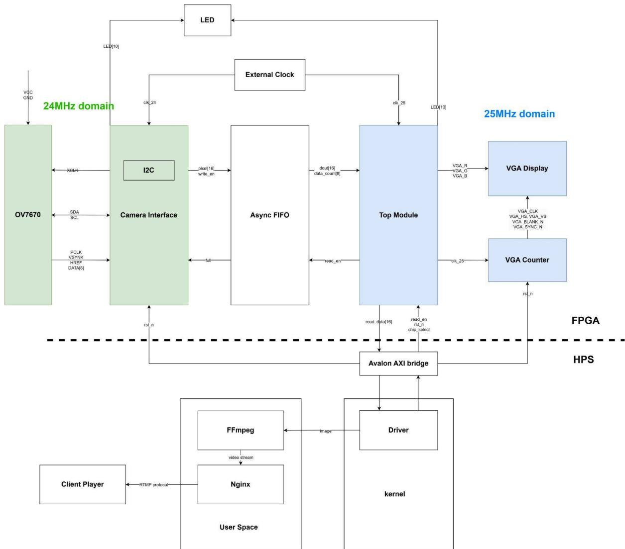
The system is generally divided into 2 parts: **FPGA** and **HPS**, which correspond to the hardware and software parts.
