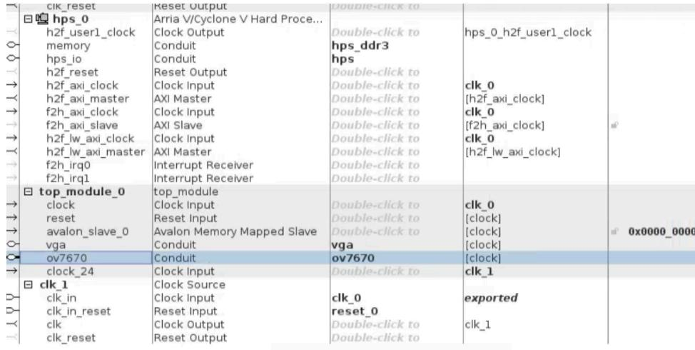
The signal we tried to transmit is under the listed format below:
