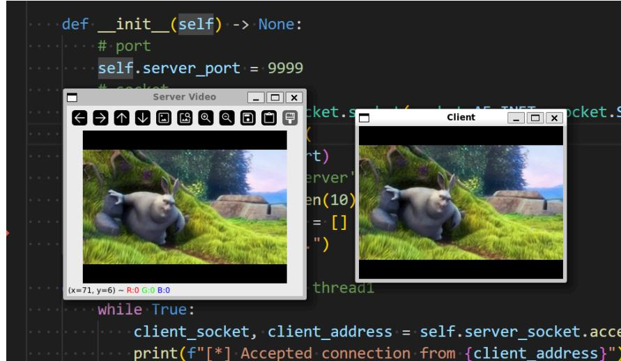
By design, the internet server should directly call the driver in the kernel module to get the video frames. But as mentioned in the “driver” section, in reality, we implement a sender, as a user program. The sender interface with the driver and sends the video frames to the server via socket. This can be redundant design but we don’t have time to change it.
