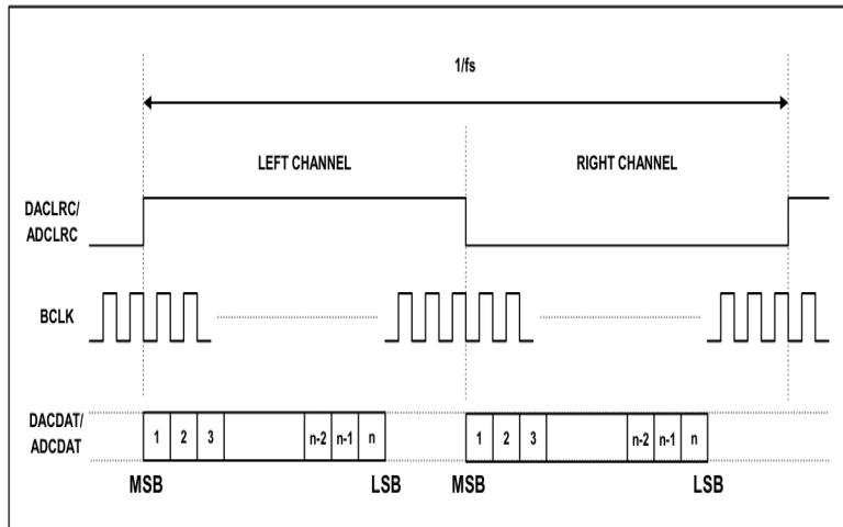
Thankfully, the CODEC Interface IP adeptly handles the intricacies of the underlying communication protocol, allowing us to focus on a select set of critical lines at the interface level: CLK, advance, ADC\_left/right, and DAC\_left/right.
