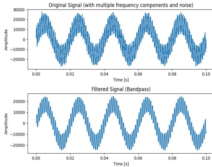
We created a testbench to evaluate our filter. The figure demonstrates that after filtering the data, the output aligns with the input data, successfully removing the undesired frequencies.
