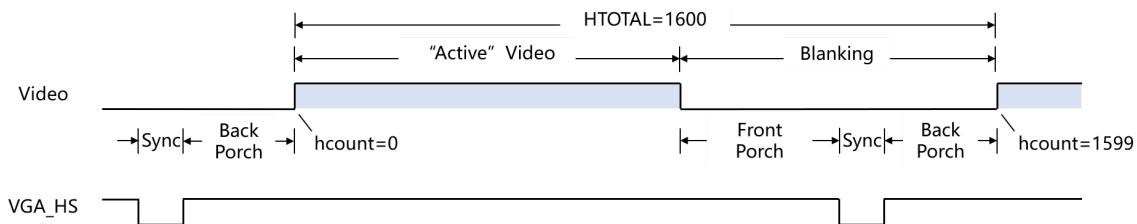
In this module, every two clk50 cycles correspond to one pixel. Every horizontal line is counted, so the vcount is incremented every time a full horizontal line completes its count. Since hcount completes one cycle every 1600 clk50 cycles, vcount is incremented once every 1600 clk50 cycles.
