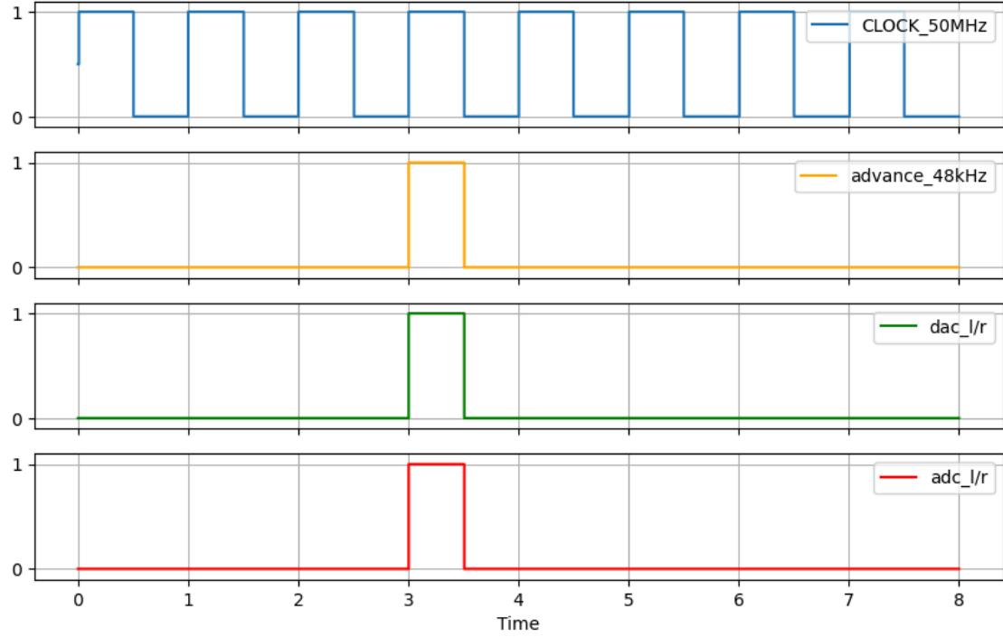
Here, all of these signals are synchronized. As the advance becomes 1, it indicates that it is ready to read the 16-bit audio input data from the microphone (ADCDAT) and send the 16-bit audio output data to the speaker (DACDAT).
