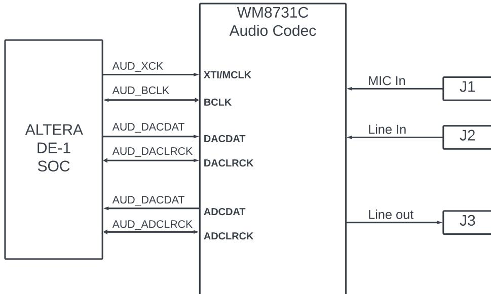
To achieve this setup, the I2C (Inter-Integrated Circuit) protocol will be utilized for programming the Audio CODEC. Analysis reveals a total of 11 distinct registers (R0 – R9, R15). Upon initial power-up, the registers reset to default values, which may not align with the desired configuration.
