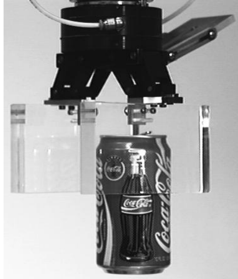
Figure 5: The image in Figure 4 after refraction compensation. The occluding boundary of the object is seen to have shifted back to its correct position.
