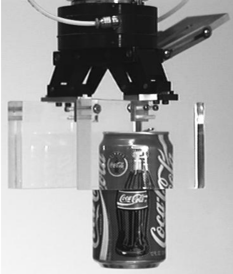
Figure 4: An object being held by a parallel-jaw transparent gripper. The image shift of the object area behind the gripper is caused by refraction.
