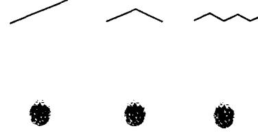
Figure 3: Phantom Surfaces: Each of the sketched surfaces would produce nearly identical texture measurements F . The only cue to differentiating between them is small perspective changes. Thus, if the first surface on the left is the true surface, than either the middle or right surface may – in presence of noise – actually minimize Eq. 4.
