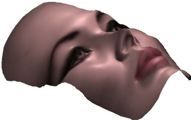
Figure 7. A texture mapped reconstruction of the mannequin face, rendered with a Phong reflectance model.
