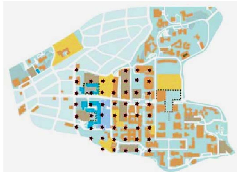
UCLA's seismic array (under construction)
