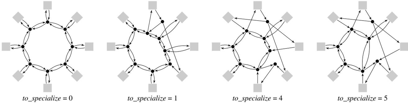
**Figure 3:** Networks produced by our algorithm employing a ring fallback for a certain system with 8 ports. More specialization steps produces a more customized network and a smaller ring.
