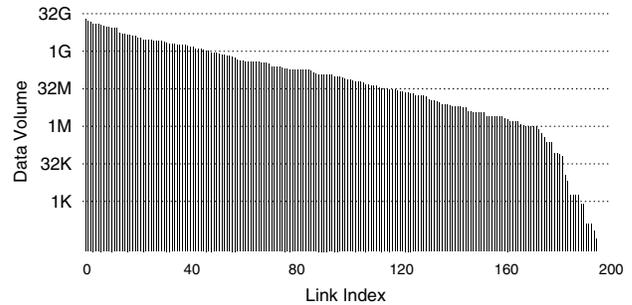
**Figure 1: Motivation for limited specialization: the volume of link traffic falls off exponentially from the busiest links, suggesting only a handful of specialized links are necessary. (TPC-H on the Q100)**
