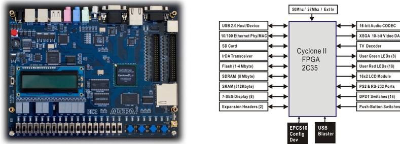
**Fig. 2.** The Terasic DE2 Board and its block diagram [1]. Ample pins on its Cyclone II FPGA enabled a star-based topology that made using external peripherals vastly easier than with the XSB, but the need for complex software for peripherals such as the USB controller was limiting.
