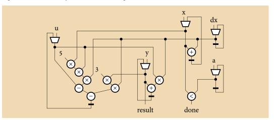
This single-cycle implementation is correct but uses a lot of multipliers. Mapping a computation to a resource-constrained datapath is a classical problem in high-level synthesis; many effective techniques for it exist. For example, Paulin et al. consider a two-multiplier datapath with an adder, subtractor, and comparator [18]. Their schedule below illustrates how to compute the function using this datapath.
