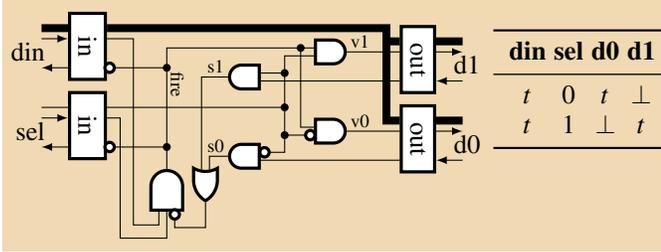
Figure 6. A *switch* block implementation and its firing rules. When tokens are present on both *din* and *sel*, the block transfers the token on *din* to *d0* or *d1* depending on the value of *sel*.
