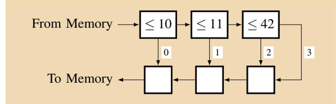
Figure 10. A range partitioning pipeline configured with splitters (10, 11, 42). Data is loaded from memory and flows right until it satisfies the predicate, then it falls, is tagged with the bucket number, and flows left to memory.
