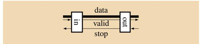
Figure 5. A single-place buffer built from a pair of our input and output buffers. This behaves like the relay station of Li et al. [13].
