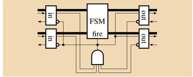
Figure 4. A two-input, two-output unit-rate dataflow block with state. The Mealy-style state machine must hold its state when  $fire$  is false. Note that the “stop” signals inside the core are active-low.
