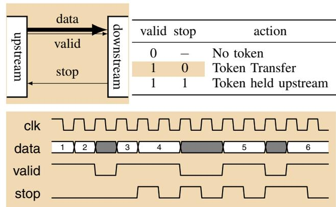
Figure 1. Our flow-control protocol transmitting the sequence of tokens 1,2,3,4,5,6. After Cortadella et al. [5] and Li et al. [13].
