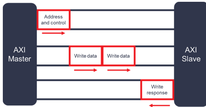
An AXI write with write addr, write data, and write resp channel
