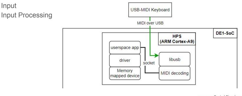
Control Singal Audio Signal Path (16bit, 48kHz) Memory Mapped Addressing
