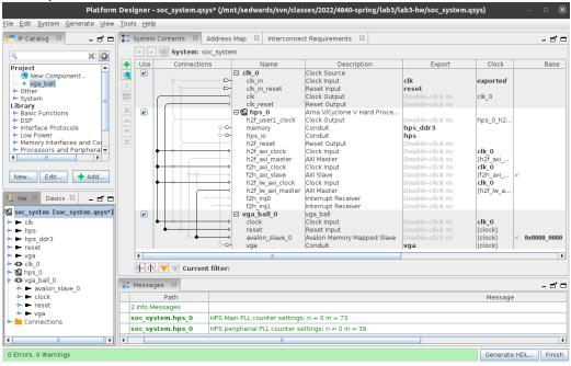
Save the system (File→Save), which should write *soc\_system.qsys*.
