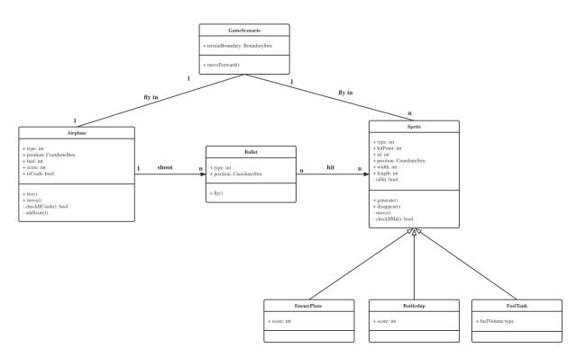
Figure 3-1 UML Class Diagram of River-Raid Project
