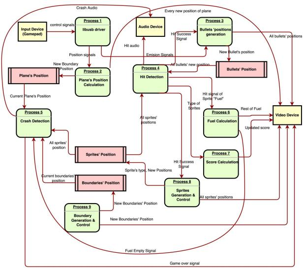
Figure 2-1 Data Flow Diagram of the Air-Raid project
