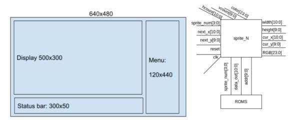
Figure 3a (left): Concept Sketch of physical display Figure 3b (right): internals of a single sprite module
