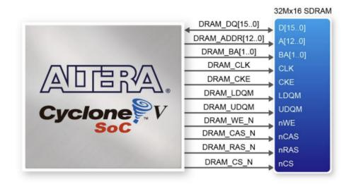
Fig 11: FPGA-SDRAM interface
