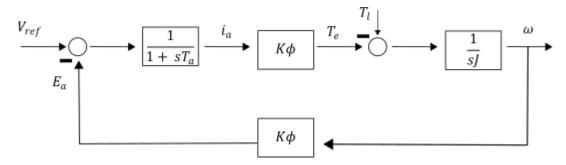
Figure 3: Block diagram of the DC motor model
