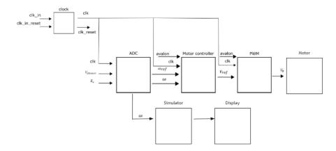
Figure 2: Block diagram of the hardware for the DC motor controller
