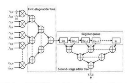
Figure 5: Convolution module. Multiplication of data and coefficients are shown for *M*th column
