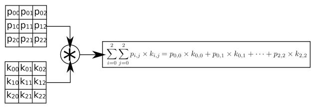
Figure 3: Convolution operation for a 3x3 kernel
