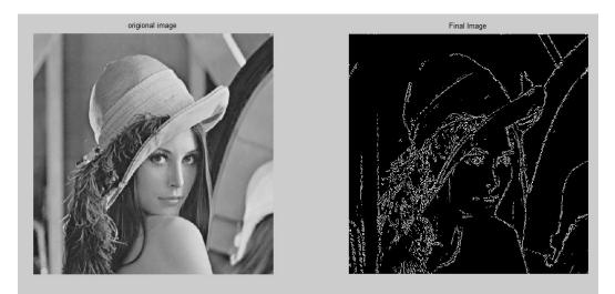
Figure 2: Effects of a Sobel filter (3x3 kernel size)
