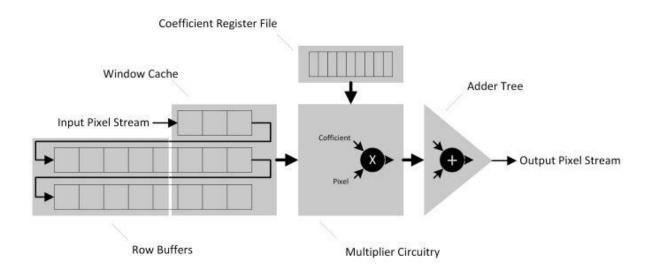
Figure 4: Image filter block diagram
