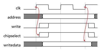
Bus cycle starts on rising clock edge Peripheral latches data two cycles later For slower peripherals
