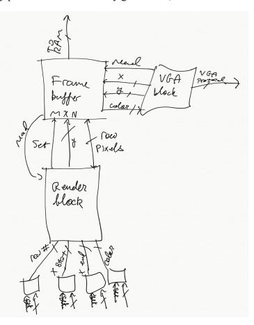
should also be minimal. As for the hardware/software interface, the plan is to have the four control registers (row number, start column, end column, and color), as well as a status bit (ready to write). The software will poll the device until it is ready to render the next row, perhaps trying to be smart about how long to wait in between polls by computing some statistics about average
