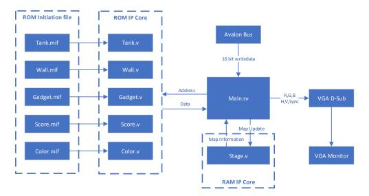
Fig.6 VGA Module Block Diagram
