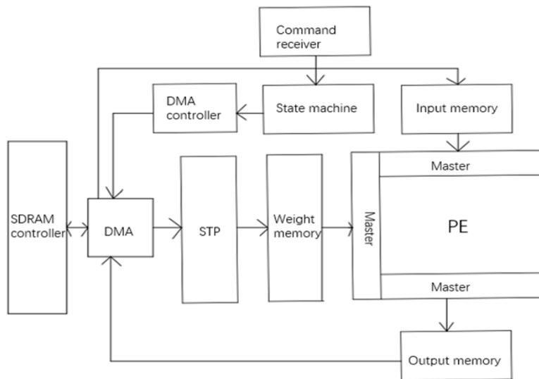
Fig 4.1 Hardware architecture
