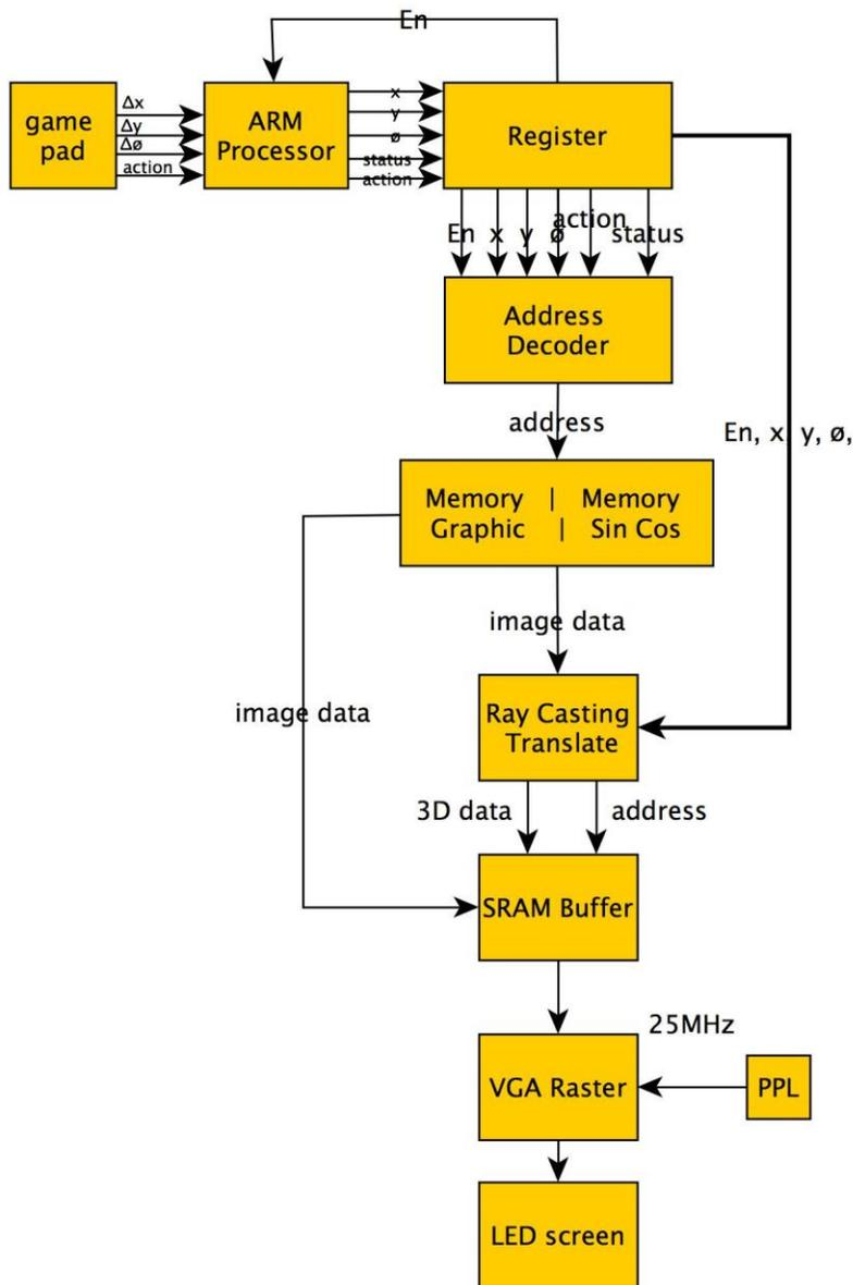
X,Y and  $\theta$  are used to build the 3D map. En signal selects between explore mode and fighting mode, referring to separated music and scenes. Also the feedback of En will decide how the controller works. There will be a delay between the scene change. Status signal refers to the attacks and hp of player, shown in the screen as 2D digits. Action signal decides what to display in the screen when the player will act when facing the enemy in the game.
