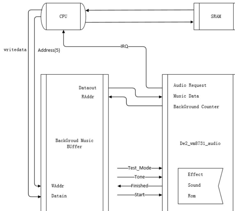
The audio controller consists of a RAM buffer for background music and Wolfson WM8371 audio codec. The buffer size is  $32 * 16$  bits. In the block diagram above, Waddr is the write address controlled by CPU, whose width is 5 bit, representing 32 entries. DataIn interface get data from CPU. Raddr is the read address controlled by audio codec counter. DataOut send data in the Raddr to the codec. When the last entry is read from the buffer, the codec sends a request to CPU ask for more data.
