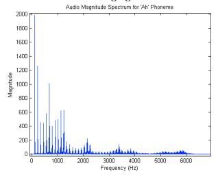
We can see from the figure that there will be a frequency component that has the largest amplitude in spectrum. We use this frequency as the fundamental frequency. And will be stored and compared with the fundamental frequency of the previous time period. Since different people have different fundamental frequency, we only use the difference across time.
