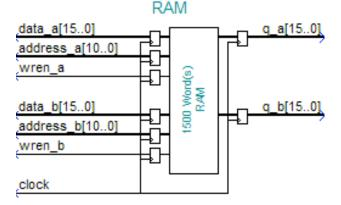
In order to deal with the asynchronous problem caused by different speed of MIC and FFT, a counter is used to generate one clock cycle write enable signal even though the data is valid during multiple clock cycles. Obviously, the clock frequency of the RAM should be identical to that of the faster device.
