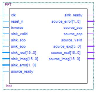
We will use the FFT IP core in Quartus. The IP core uses the N complex vector in the time domain as the input, and outputs the complex vector in the frequency domain in the natural order. The inputs include 1 bit clk, 1bit reset\_n signal, 1bit inverse bit to determine the order of output, 1 bit sink valid to determine the valid bit of the input, 1 bit start of packet signal, 1bit end of packet signal, one 16 bits real part of signal, one 16 bits imaginary part of signal, 2
