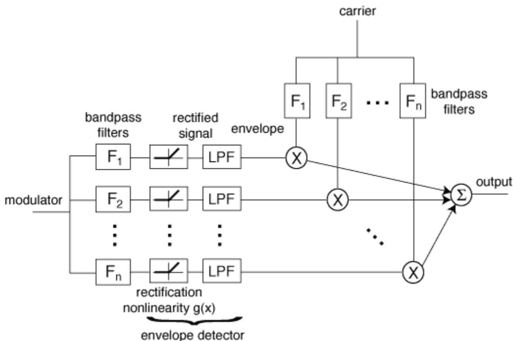
**Figure 9** – A diagram representing how a channel vocoder works.
