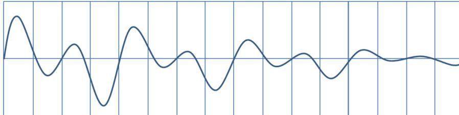
**Figure 6.** Example output signal of FM operator: the output of figure 1 with a decaying envelope which decreases the amplitude of the signal over time.
