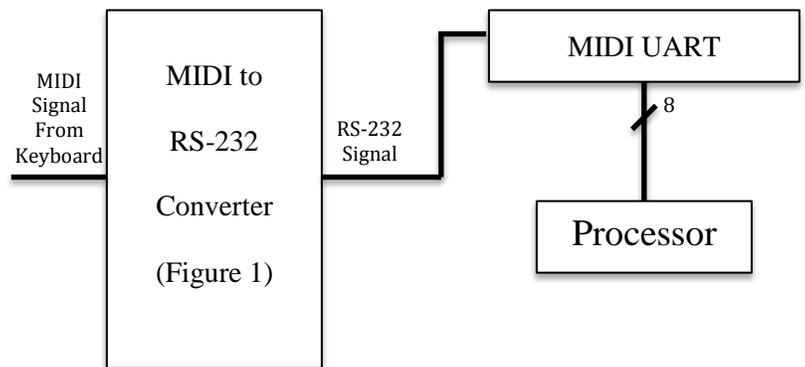
Figure 2. Block diagram for the MIDI input interface
