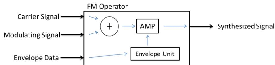
**Figure 5.** Diagram of FM operator.
