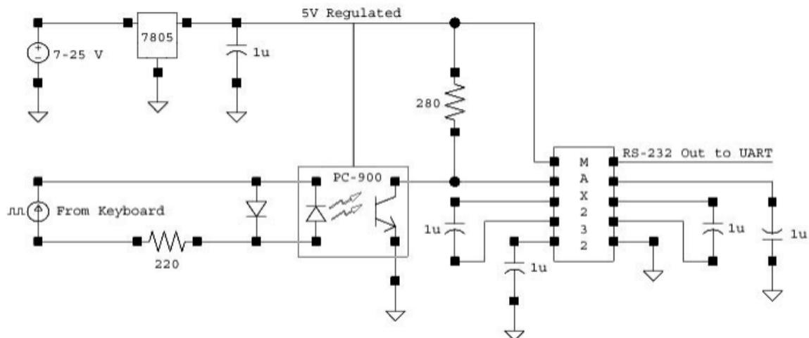
Figure 1. MIDI-in to RS-232 Conversion circuit
