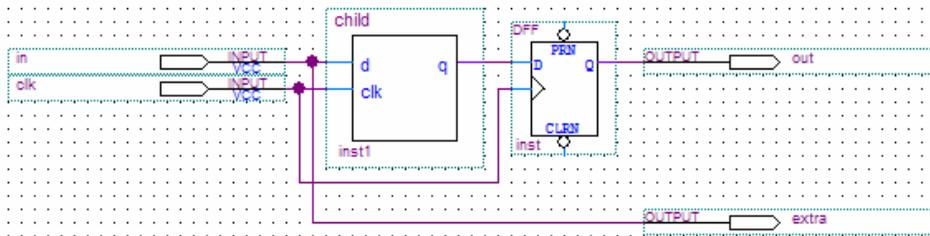
In this case, the software does not perform input register packing. If there is a Fast Input Register assignment on pin `in`, the software issues a warning that the Fitter cannot pack the node to an I/O pin because the node and the I/O cell are connected across a design partition boundary.
