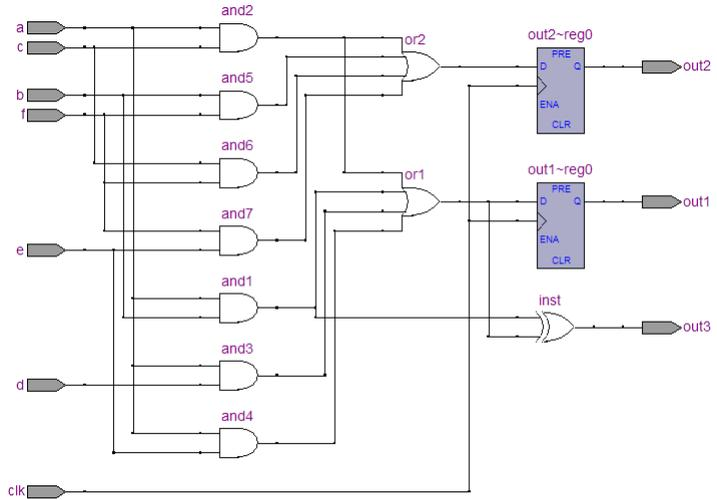
**Figure 12–17. Schematic After Combinational Logic Grouping**
