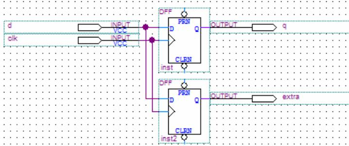
Figure 2-20. Modified Top-Level Design from Figure 2-18 Connecting Two Output Ports to Output Pins
