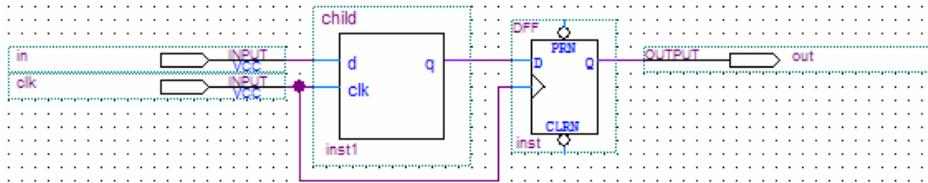
The Quartus II software performs cross-partition register packing if there is a Fast Input Register assignment on pin in. This type of cross-partition output register packing is permitted because the port interface of the subdesign partition does not have to be changed and the partition port is fed by an input pin directly.
