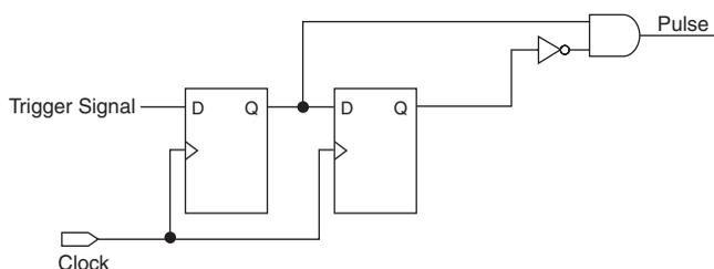
In this design, the pulse width is always equal to the clock period. This pulse generator is predictable, can be verified with timing analysis, and is easily moved to other architectures, devices, or speed grades.
