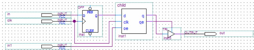
In this case, the software cannot perform register packing. If there is a Fast Output Register or Fast Output Enable Register assignment on pin out, the software issues a warning that the Fitter cannot pack the node to an I/O pin because the node and the I/O cell are connected across a design partition boundary.
