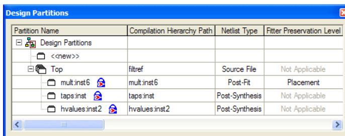
Alternatively, you can use the list of instances under the **Hierarchy** tab in the **Project Navigator** to create and delete design partitions. Right-click on an instance in the **Project Navigator** and click **Set as Design Partition**.
