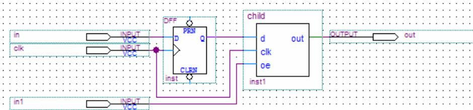
The Quartus II software performs cross-partition register packing if there is a Fast Output Register assignment, Fast Output Enable Register assignment, or both, on pin out. This kind of cross-partition output register packing is permitted because the port interface of the subdesign partition does not need to be changed, no logic needs to be optimized across the partition boundary, and the partition port feeds an output pin directly.
