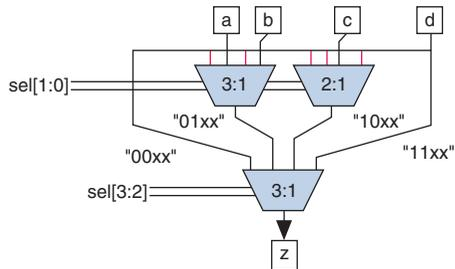
Implementing this version of the multiplexer still requires at least five 4-input LUTs, two for each of the remaining 3:1 multiplexers and one for the 2:1 multiplexer. This design selects an output from only four inputs, a 4:1 binary multiplexer can be implemented optimally in two LUTs, so this degenerate multiplexer tree reduces the efficiency of the logic.
