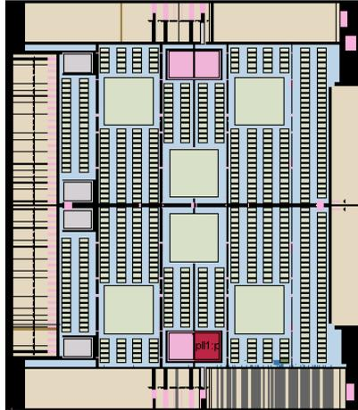
In this small example design, the logic is placed near the bottom edge. You can see the placement of a DSP block constructed of HCell Macros, various logic HCell Macros, and an M4K memory block. A labeled close-up view of this region is shown in Figure 4–16.
