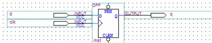
**Figure 2–33. Top-level Design Instantiating the Subdesign in Figure 2–32 as an Input Register with an Inverted Input Pin**
