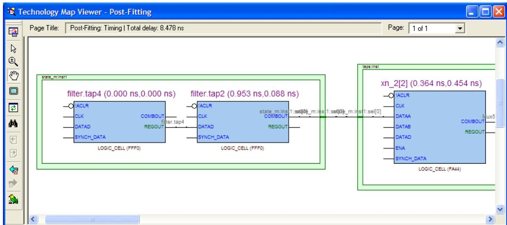
In the RTL Viewer, the schematic page displays the nodes in the path(s) between the source and destination registers with a summary of the total delay.
