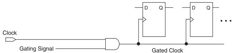
You can use gated clocks to reduce power consumption in some device architectures by effectively shutting down portions of a digital circuit when they are not in use. When a clock is gated, both the clock network and the registers driven by it stop toggling, thereby eliminating their contributions to power consumption. However, gated clocks are not part of a synchronous scheme and therefore can significantly increase the
