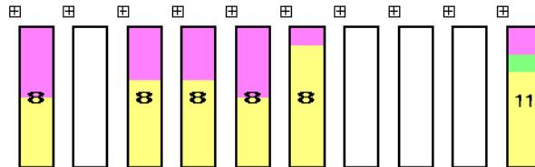
The Field view is a color-coded, high-level view of your device resources that hides both cell and LAB details. In the Field view, you can see critical paths and routing congestion in your design.
