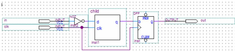
**Figure 2–34. Top-level Design Instantiating the Subdesign in Figure 2–33 as an Output Register Feeding an Inverted Output Pin**
