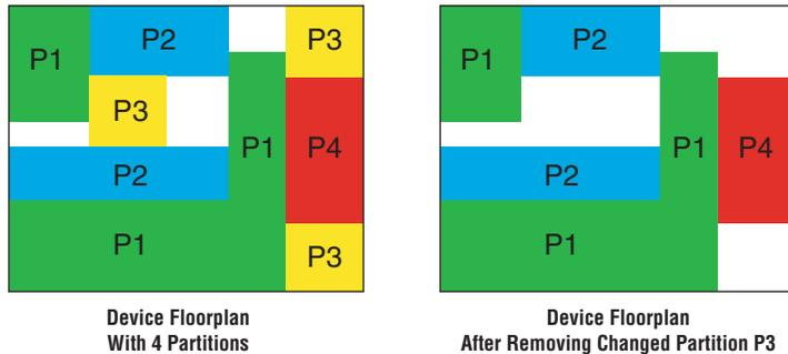
Performing this placement is very difficult. The Fitter may not be able to find any legal placement for the logic in partition P3, even if it was able to do so in the initial compilation. If the Fitter does find a legal placement, the results are probably sub-optimal.
