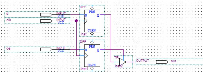
**Figure 2–22. Top-level Design Instantiating the Subdesign in Figure 2–21**
