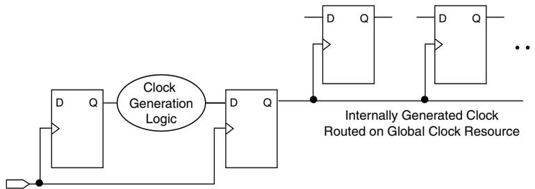
Registering the output of combinational logic ensures that the glitches generated by the combinational logic are blocked at the data input of the register.
