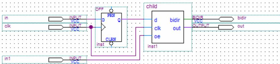
The Quartus II software performs cross-partition register packing if there is a Fast Output Register, Fast Output Enable Register, or Fast Input Register assignment on pin `bidir`. This type of cross-partition output register packing is permitted because the port interface of the subdesign partition does not need to be changed and the partition port feeds a bidirectional pin directly.
