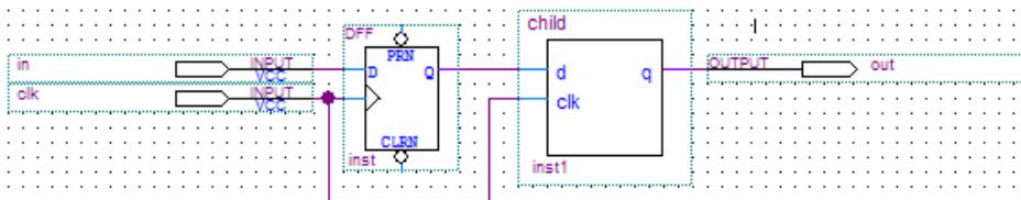
The Quartus II software performs cross-partition register packing if there is a Fast Output Register assignment on pin out. This type of cross-partition output register packing is permitted because the port interface of the subdesign partition does not need to be changed and the partition port feeds an output pin directly.
