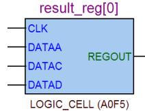
To view the contents of one or more atom primitive instances, select the desired atom instances. Right-click a selected instance and click **Display Content**. You can also double-click on the desired atom instance to view the contents. Figure 12-8 shows an expanded version of the instance in Figure 12-7.
