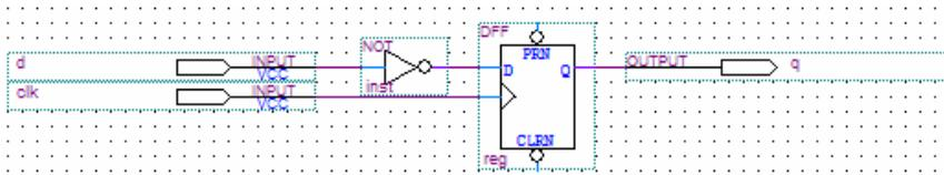
**Figure 2–31. Top-level Design Instantiating the Subdesign in Figure 2–30 as an Input Register**
