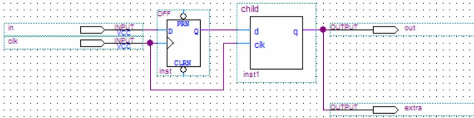
In this case, the software does not perform output register packing. If there is a Fast Output Register assignment on pin out, the software issues a warning that the Fitter can't pack the node to an I/O pin because the node and the I/O cell are connected across a design partition boundary.
