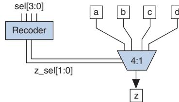
The design for the recoder can be implemented in two LUTs and the efficient 4:1 binary multiplexer uses two LUTs, for a total of four LUTs. The original degenerate multiplexer required five LUTs, so the recoded version uses 20% less logic than the original.
