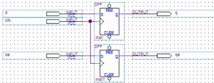
**Figure 2–24. Top-level Design Instantiating the Subdesign in Figure 2–23 to Drive Output Enable Logic**
