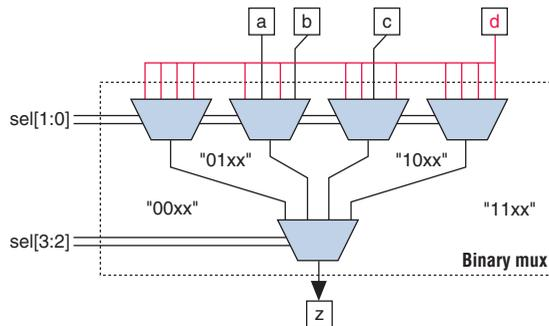
In the example in Figure 6–4, the first and fourth multiplexers in the top level can easily be eliminated because all four inputs to each multiplexer are the same value, and the number of inputs to the other multiplexers can be reduced, as shown in Figure 6–5.
