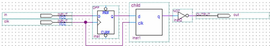
In these cases, the software does not perform register packing. If there is a Fast Input Register assignment on pin `in` in Figure 2–33 or a Fast Output Register assignment on pin `out` in Figure 2–34, the software issues a warning that the Fitter cannot pack the node to an I/O pin because the node and the I/O cell are connected across a design partition boundary.
