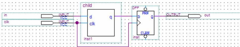
The Quartus II software performs cross-partition register packing if there is a Fast Input Register assignment on pin `in`. This kind of cross-partition input register packing is permitted because the software can implement the logic for the inversion with the input register inside the partition, and then the partition port is fed by an input pin directly.
