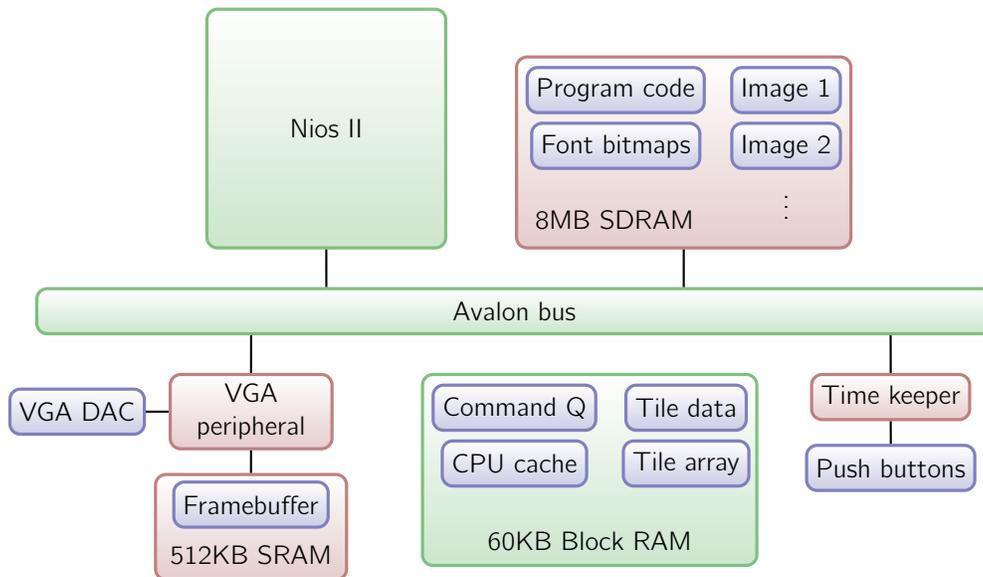
Figure 2: Overview of the components of the device
