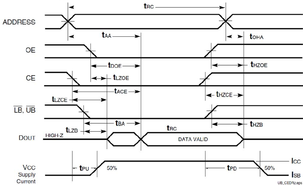
Figure 1 - Timing Diagram for SRAM read
