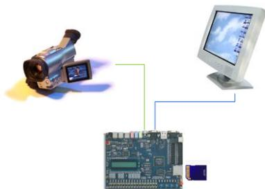
For this design we plan to use the NIOS process along with several Avalon peripherals. The system will perform 2 basic operations; the first is to display the video input to the VGA output, and the second is to compress a single frame and save it to a file in the SD card. The first operation requires to convert the analog input to digital and change the color space. Then the video signal is sent to the VGA controller to
