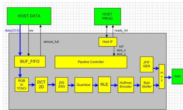
The output of this module is saved to memory. Inside, this core has a complex Finite State Machine, that keeps track of the current hardware operation. The NIOS processor can orchestrate when is module is invoked, so that the output will be saved to a file in the SD card. This module is based on project *mkjpeg* from [opencores.org](http://opencores.org).
