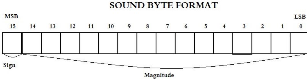
The most significant bit of the sound byte is the sign bit. If this bit is 0 (positive number), then the resulting integer sent to the software ranges from 0 to 32,767 in order of increasing magnitude. If it is 1 (negative), then the integer ranges from 32,768 to 65,535 in decreasing magnitude, as a two's complement system is used. This relation of the physical bits in the sound byte to the integer passed to the software will be important for the frequency algorithm implemented in the software.
