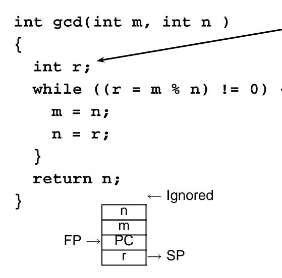
Automatic variable Allocated on stack when function entered, released on return Parameters & automatic variables accessed via frame pointer Other temporaries
