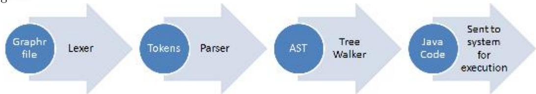
For the user's convenience, we have constructed a tool which performs the above steps and then executes the Java program using the Java Runtime Environment (described as a requirement in section 1.2) installed on the user's computer.
