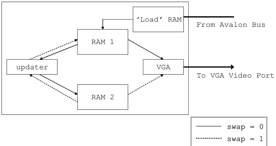
The vga\_raster in essence serves three functions. The first is to accept the initial conditions from the Nios Processor across the Avalon bus. The second is to take the current state of the board and output it to the screen through the 'VGA' block. The last, but equally important job of the vga\_raster is to update the current state of the board and output the next generation to another block of RAM.
