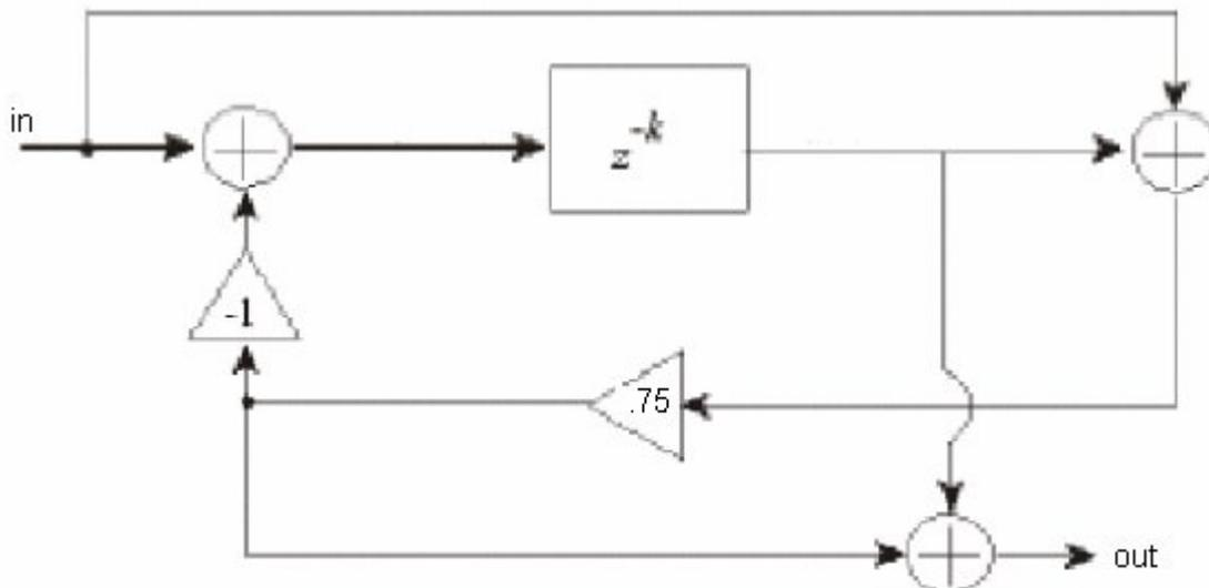
Our first stage used  $k=2048$  (about 1/20 of a second), and our second stage used  $k=5376$  (about 1/10 of a second). The sizes of the delays may be easily adjusted in the constant declarations; this adjusts the duration of the reverberations. We had a lot of fun experimenting with this. The second stage echoes the echoes generated by the first stage, producing a more natural sounding output.
