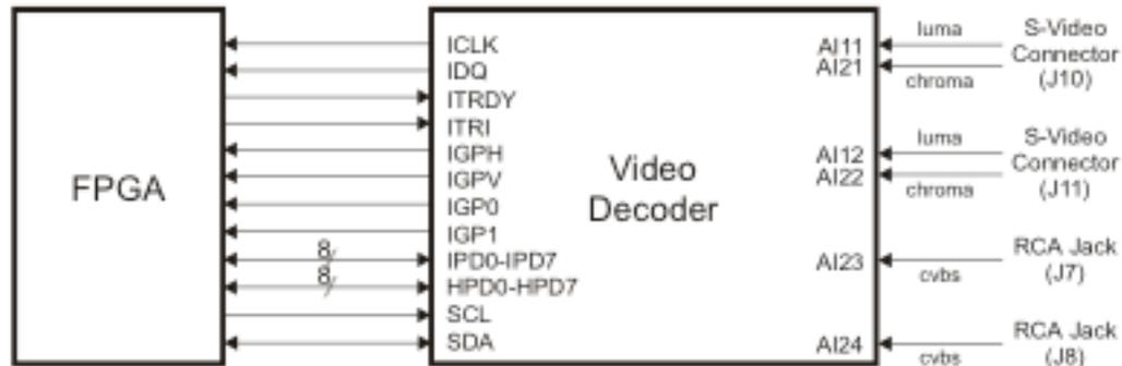
Video arrives at the FPGA over two eight bit buses. The IDP bus is for luminance values (Y) and the HDP bus is for chrominance values (UV).
