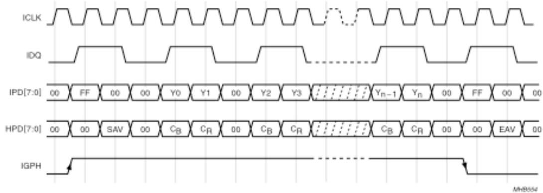
This timing diagram shows the beginning and end of a line. SAV means Start Active Video and EAV means End Active Video. The diagram shows the role played by IDQ and IPGH. IPGH indicates the beginning and end of each active line.
