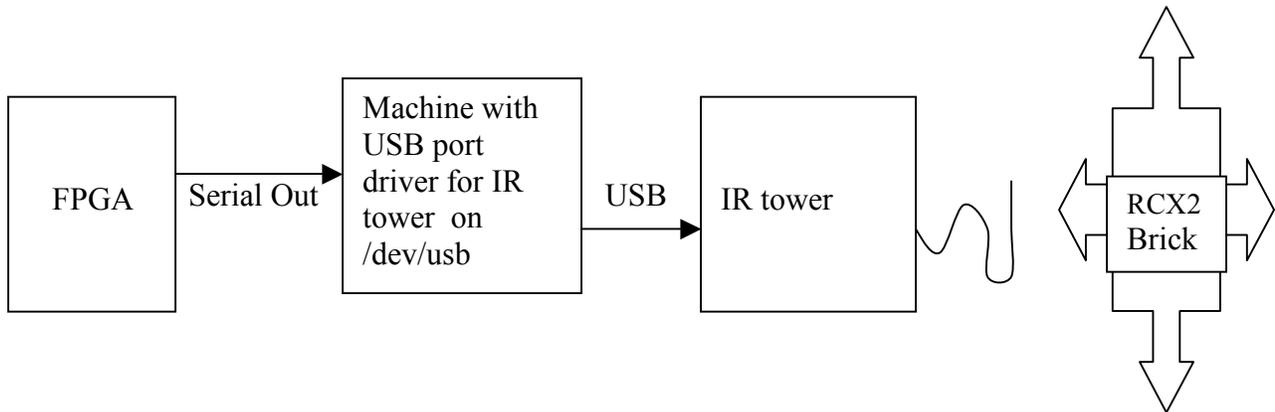
We use the Lego mindstorm robot to implement our directional cues. The computer for the mindstorm is called the RCX2, or the brick. The block diagram above shows the main components in the robot communication system.
