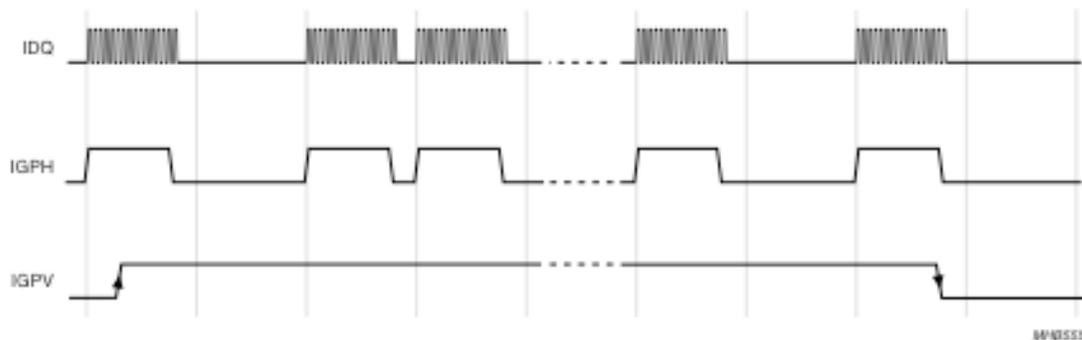
This timing diagram shows the role of the IPGV signal. It indicates the beginning and end of each frame. Also, we see that IDQ is constantly going on and off in the middle of active video lines.
