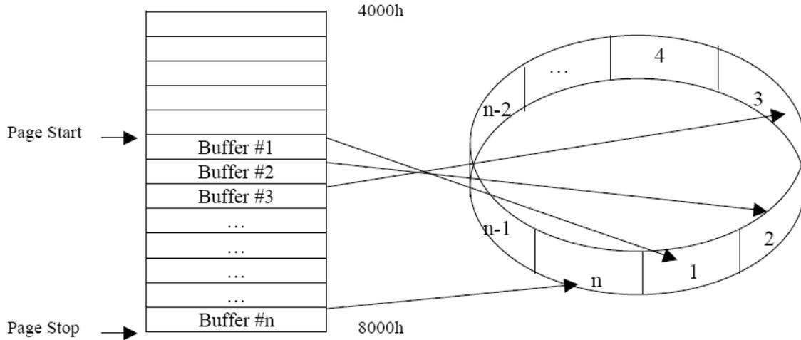
**Figure (2) FPGA To SRAM Block Diagram**
