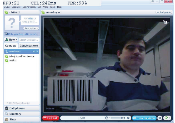
Figure 3: Screen shot of vDelay-R application. FPS, CDL, and FRR statistics are shown at the top of the image. The barcode received from the caller user agent is also visible.
