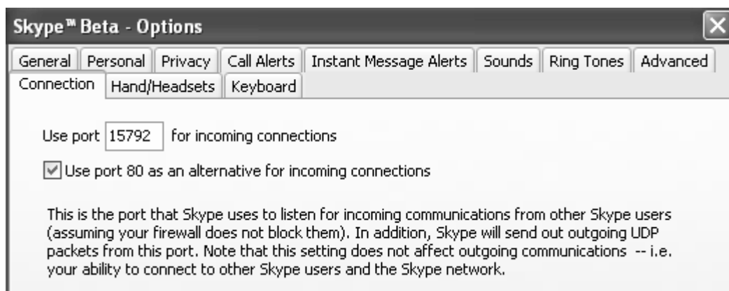
Figure 16. Skype connection tab. It shows the ports on which Skype listens for incoming connections.
