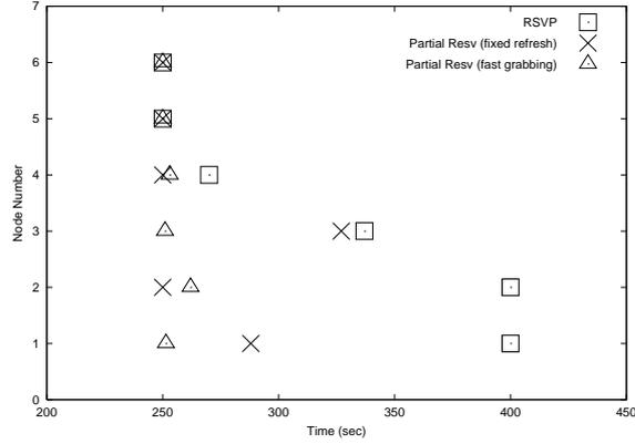
Figure 5. Reservation sequence for RSVP, YESSIR (retry with only refresh), and YESSIR (retry whenever resource becomes available). The ordinate shows the node number in the simulation network of Figure 1.
