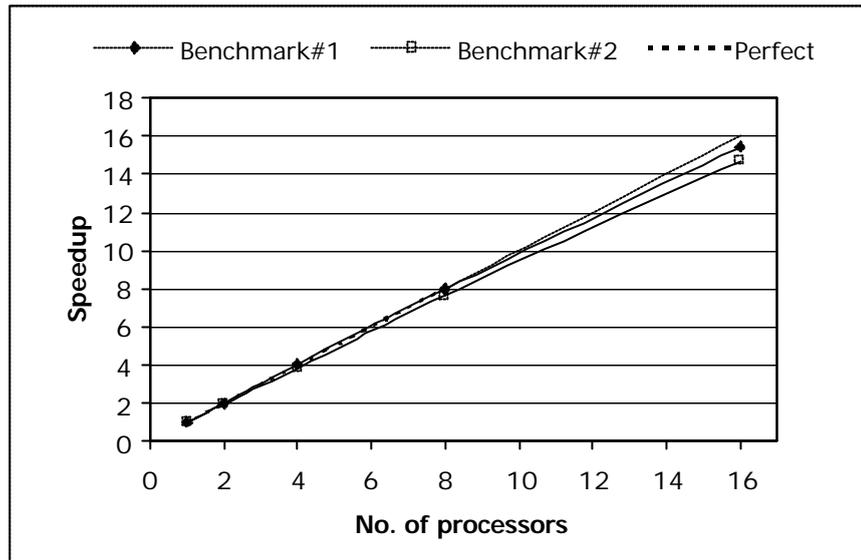
Figure 4: Performance of both benchmarks on a Linux based PC cluster, with fast Ethernet.
