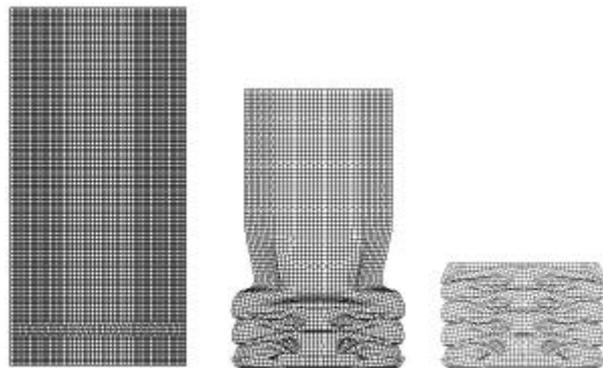
Figure 2: Crushing of octagonal steel girder
