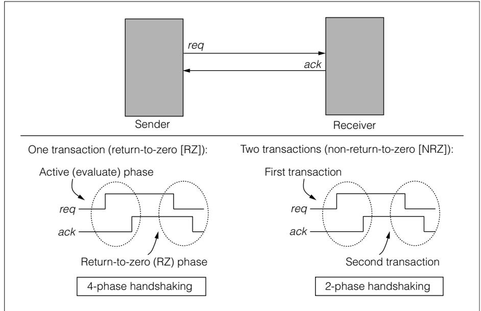
**Figure 2. Basic asynchronous communication protocols: four-phase and two-phase.**
