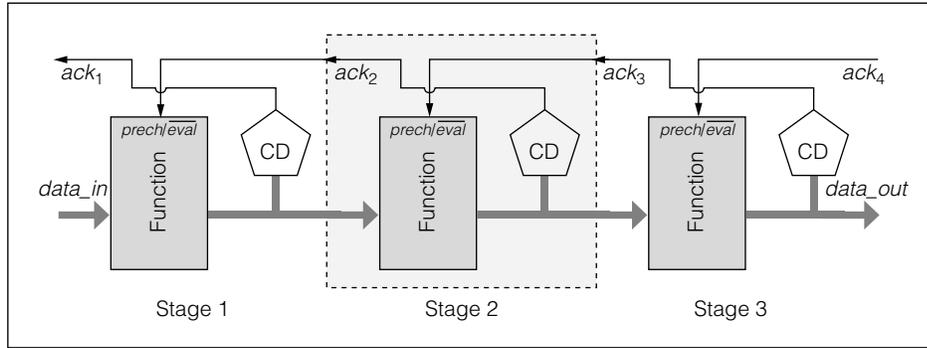
**Figure 6. Classic dynamic-pipeline style: Williams and Horowitz' PSO pipeline. (CD: completion detector.)**
