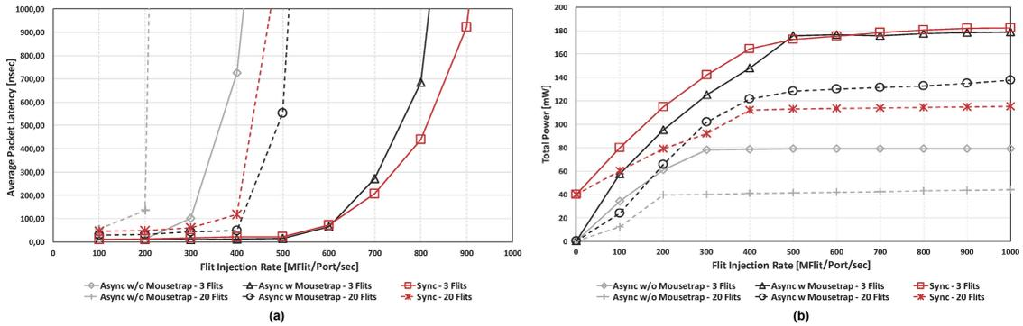
FIGURE 3. Comparative network evaluation. (a) Load curves. (b) Power consumption.
