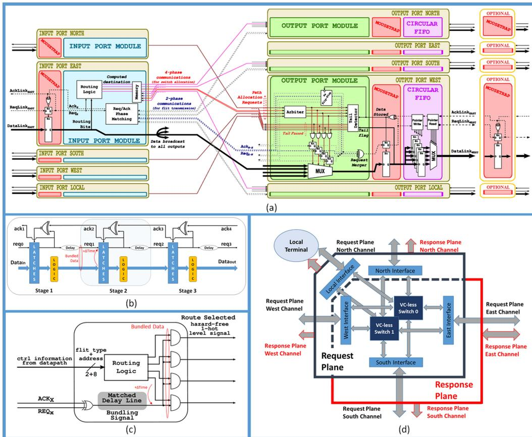
**FIGURE 1.** Proposed asynchronous switch architecture. (a) Schematic view. (b) Mousetrap asynchronous pipeline. (c) Routing logic. (d) Switch instance (2 planes, 2 VCs/plane).
