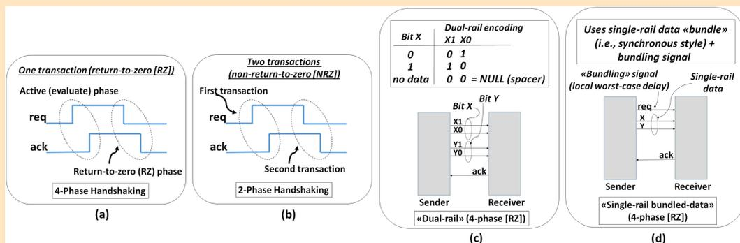
FIGURE S1. Asynchronous (a-b) handshaking protocols, and (c-d) data-encoding schemes.
