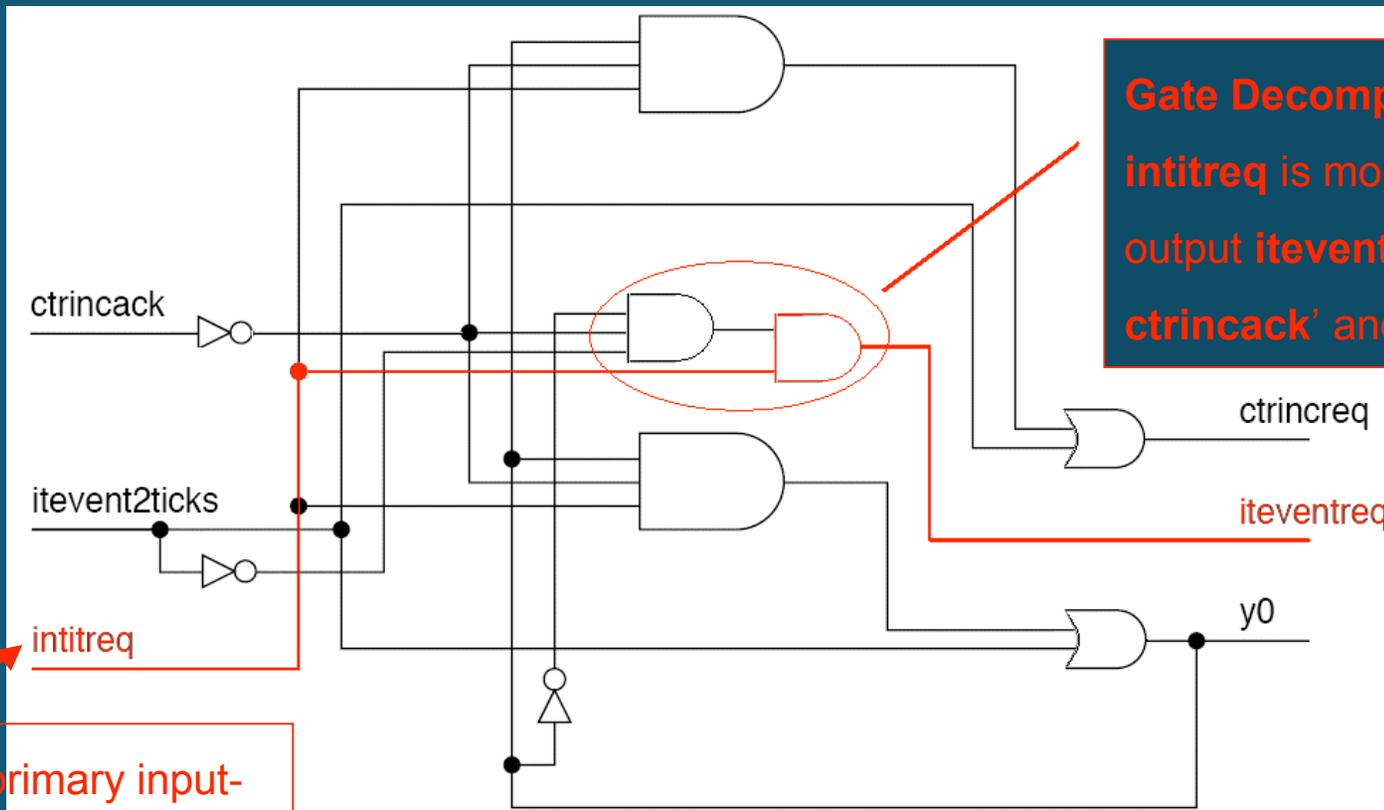
Gate Decomposed. Input `intitreq` is more critical to output `iteventreq` than `ctrincack'` and `y0'`
