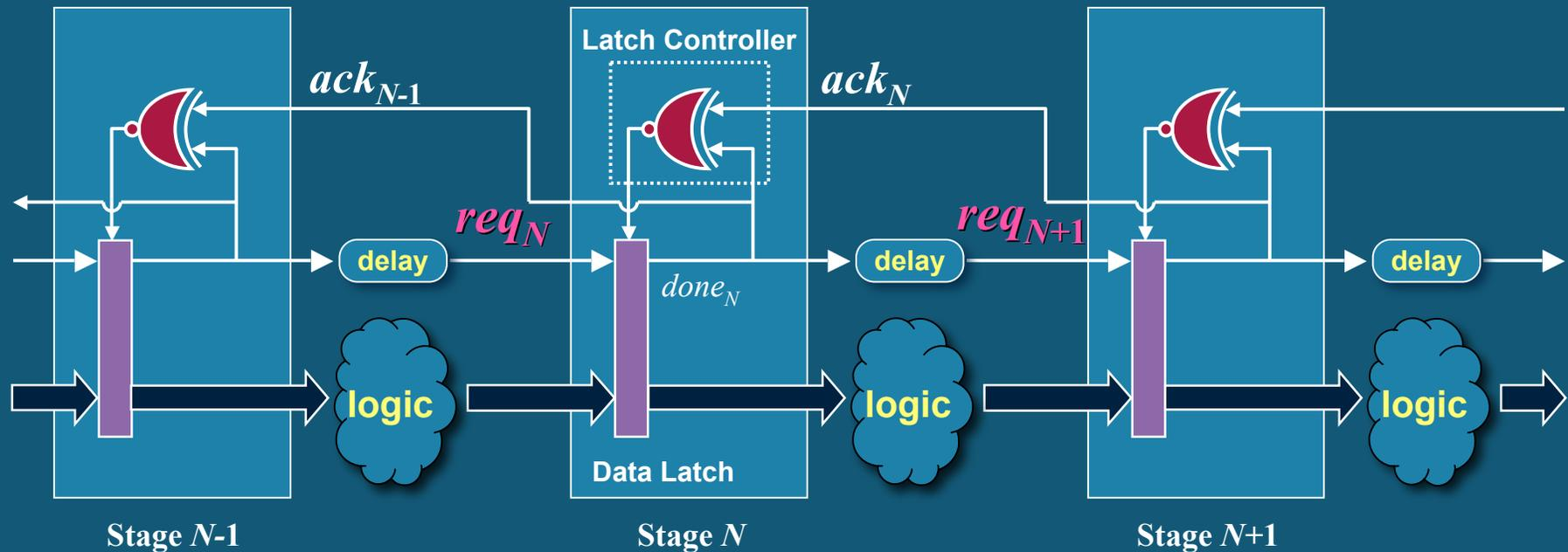
Function Blocks: use “synchronous” single-rail circuits (not hazard-free!)
