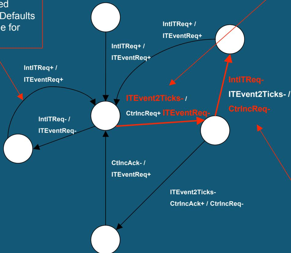
**Case 2: Some outputs colored, some outputs not.** Both user-specified data and automated approaches are used to determine criticality. **ITReventReq** will use user-specified data to determine criticality. **CtrlIncReq** will default to automated mode to determine criticality.
