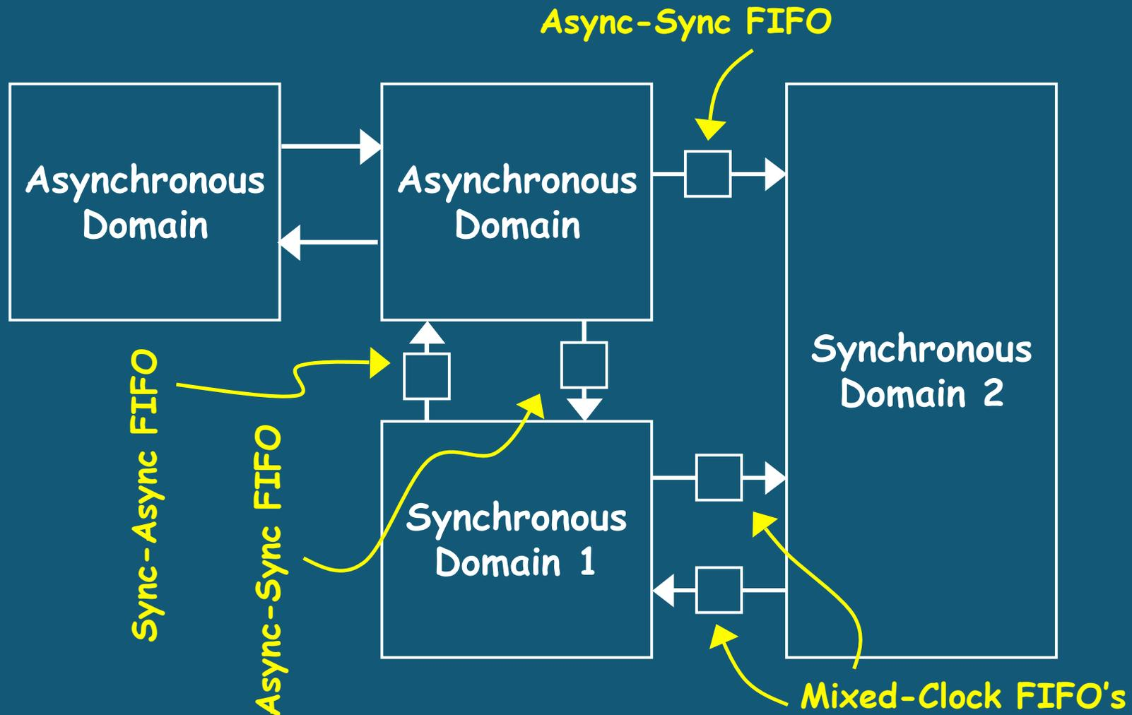
**Solution:** insert mixed-timing FIFO's  $\Rightarrow$  provide safe data transfer
