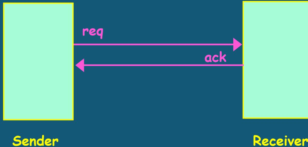
2-Phase Handshaking = "Transition-Signalling"
