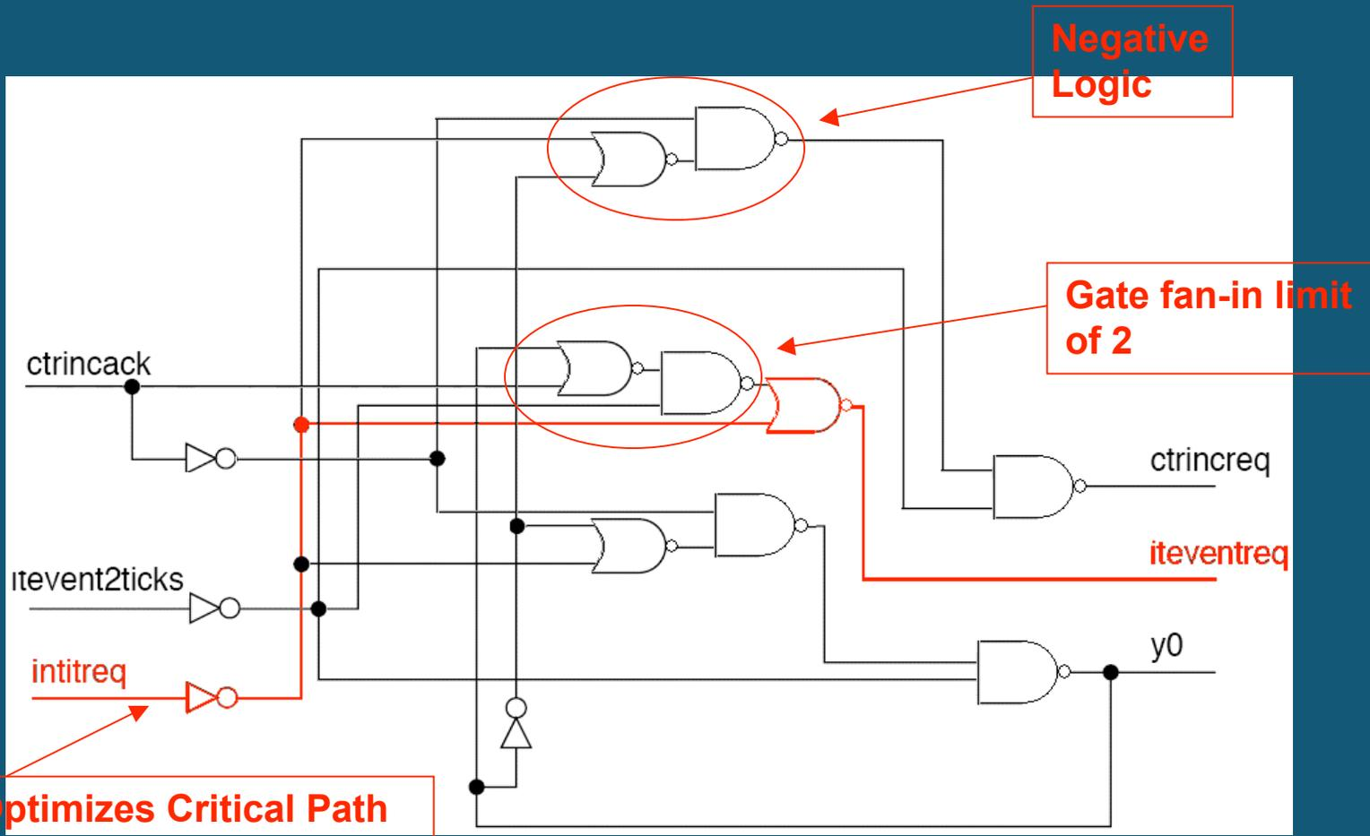
Result of MLO: Multi-Level Circuit with **negative logic**, **AND gate fan-in limit of 2**, and **CEO**.
