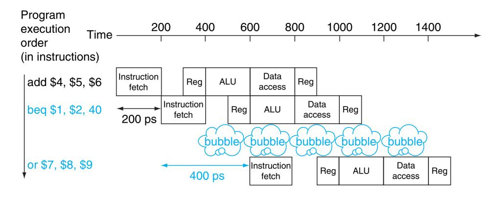
FIGURE 4.31 Pipeline showing stalling on every conditional branch as solution to control
