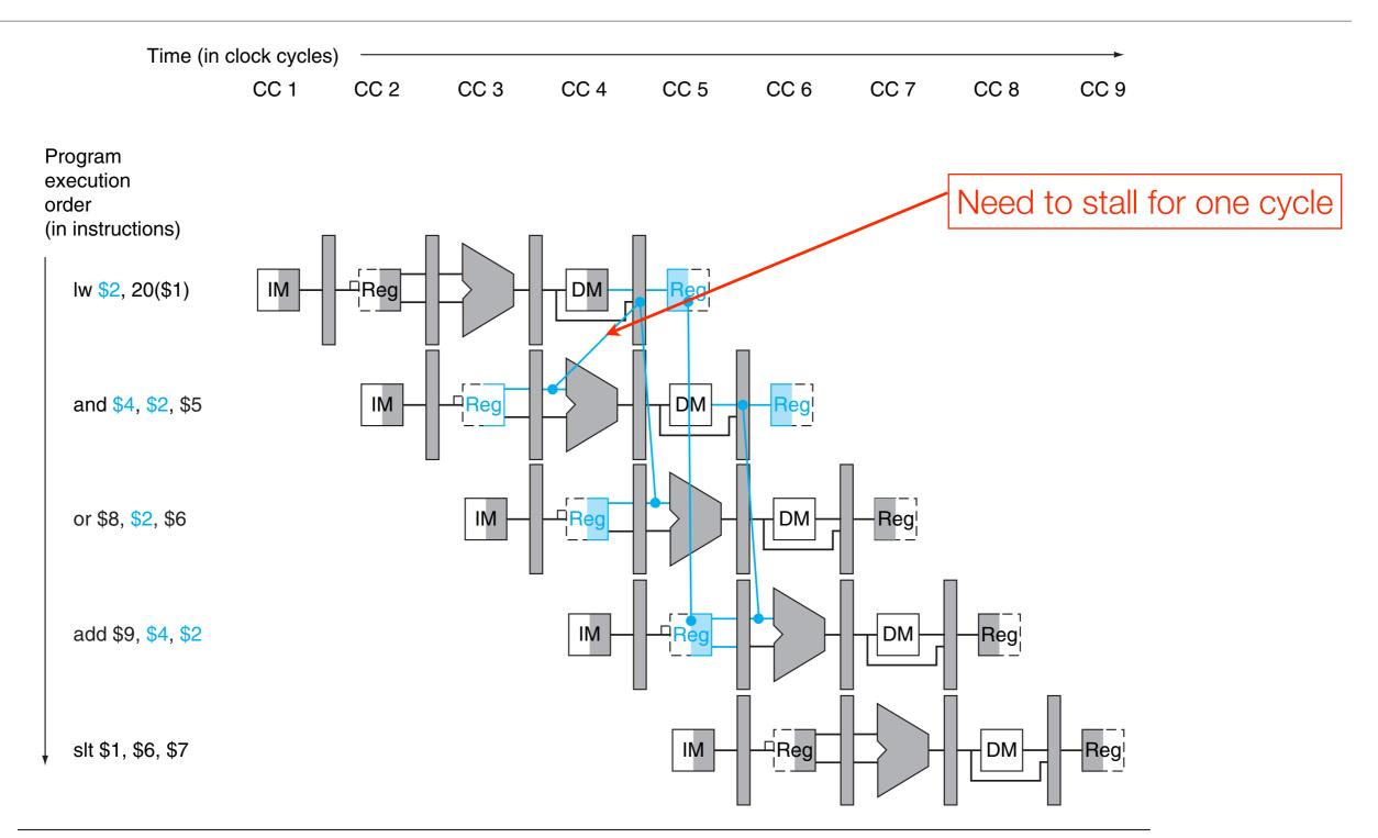
**FIGURE 4.58** A pipelined sequence of instructions. Since the dependence between the load and the following instruction (and) goes backward in time, this hazard cannot be solved by forwarding. Hence, this combination must result in a stall by the hazard detection unit. Copyright © 2009 Elsevier, Inc. All rights reserved.
