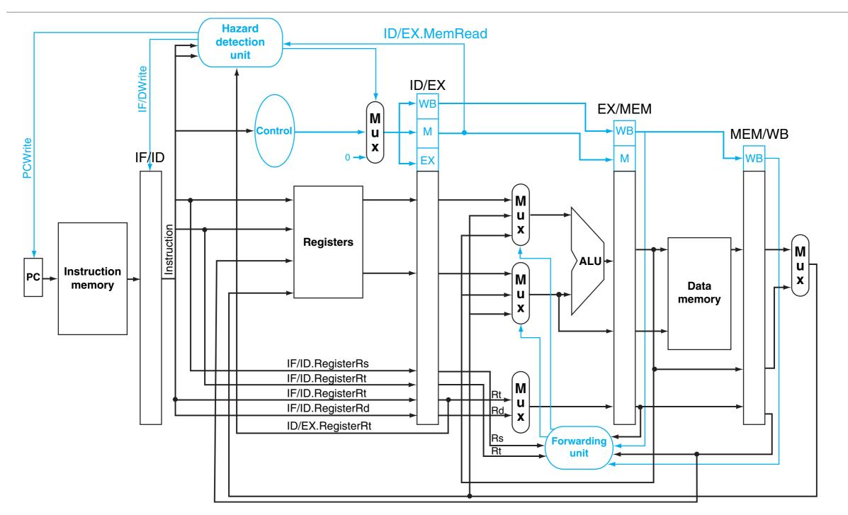
**FIGURE 4.60** Pipelined control overview, showing the two multiplexors for forwarding, the hazard detection unit, and the forwarding unit. Although the ID and EX stages have been simplified—the sign-extended immediate and branch logic are missing—this drawing gives the essence of the forwarding hardware requirements. Copyright © 2009 Elsevier, Inc. All rights reserved.
