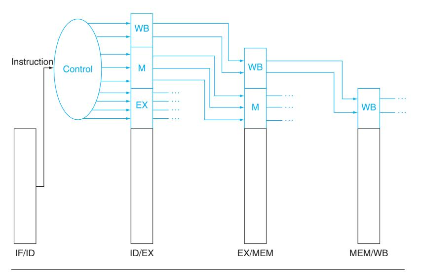
**FIGURE 4.50** The control lines for the final three stages. Note that four of the nine control lines are used in the EX phase, with the remaining five control lines passed on to the EX/MEM pipeline register extended to hold the control lines; three are used during the MEM stage, and the last two are passed to MEM/WB for use in the WB stage. Copyright © 2009 Elsevier, Inc. All rights reserved.
