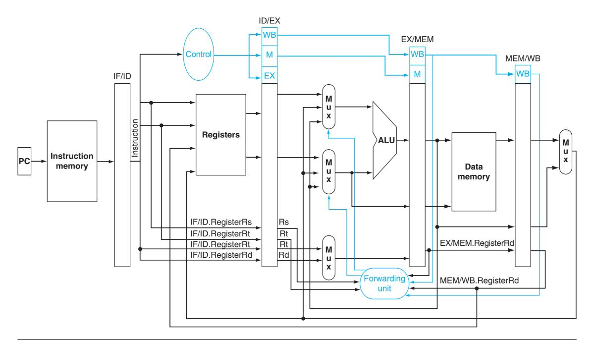
**FIGURE 4.56** The datapath modified to resolve hazards via forwarding. Compared with the datapath in Figure 4.51, the additions are the multiplexors to the inputs to the ALU. This figure is a more stylized drawing, however, leaving out details from the full datapath, such as the branch hardware and the sign extension hardware. Copyright © 2009 Elsevier, Inc. All rights reserved.
