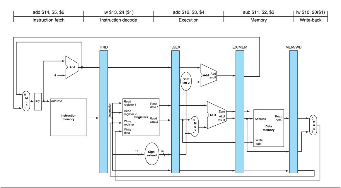
**FIGURE 4.45** The single-clock-cycle diagram corresponding to clock cycle 5 of the pipeline in Figures 4.43 and 4.44. As you can see, a single-clock-cycle figure is a vertical slice through a multiple-clock-cycle diagram. Copyright © 2009 Elsevier, Inc. All rights reserved.
