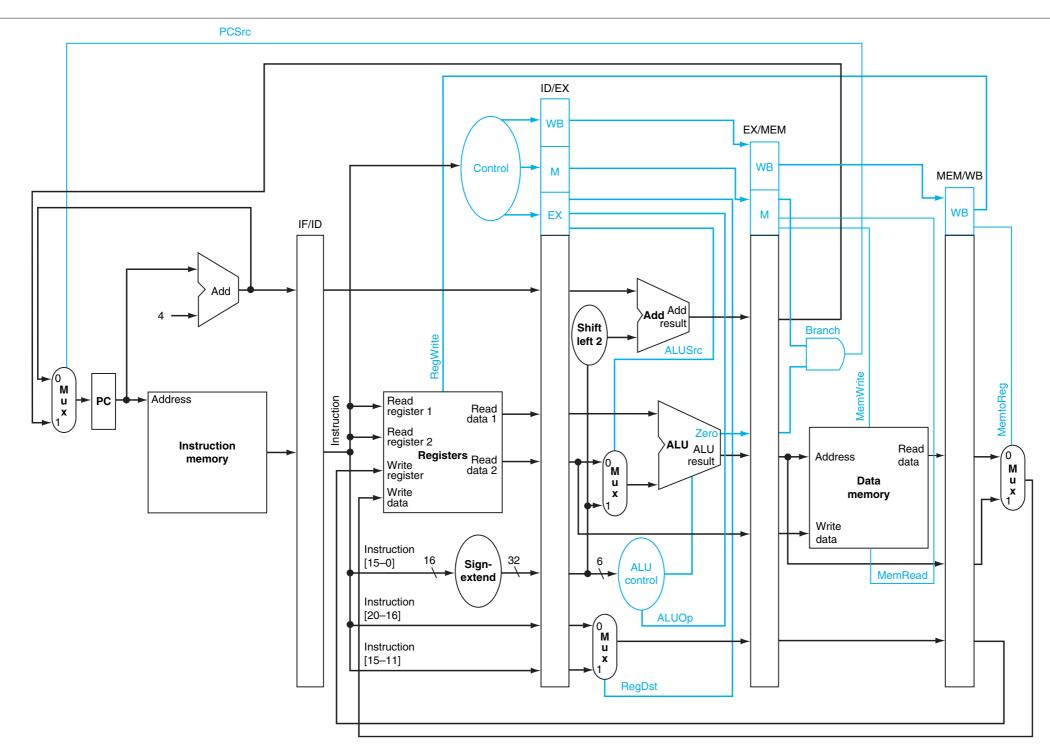
**FIGURE 4.51** The pipelined datapath of Figure 4.46, with the control signals connected to the control portions of the pipeline registers. The control values for the last three stages are created during the instruction decode stage and then placed in the ID/EX pipeline register. The control lines for each pipe stage are used, and remaining control lines are then passed to the next pipeline stage. Copyright © 2009 Elsevier, Inc. All rights reserved.
