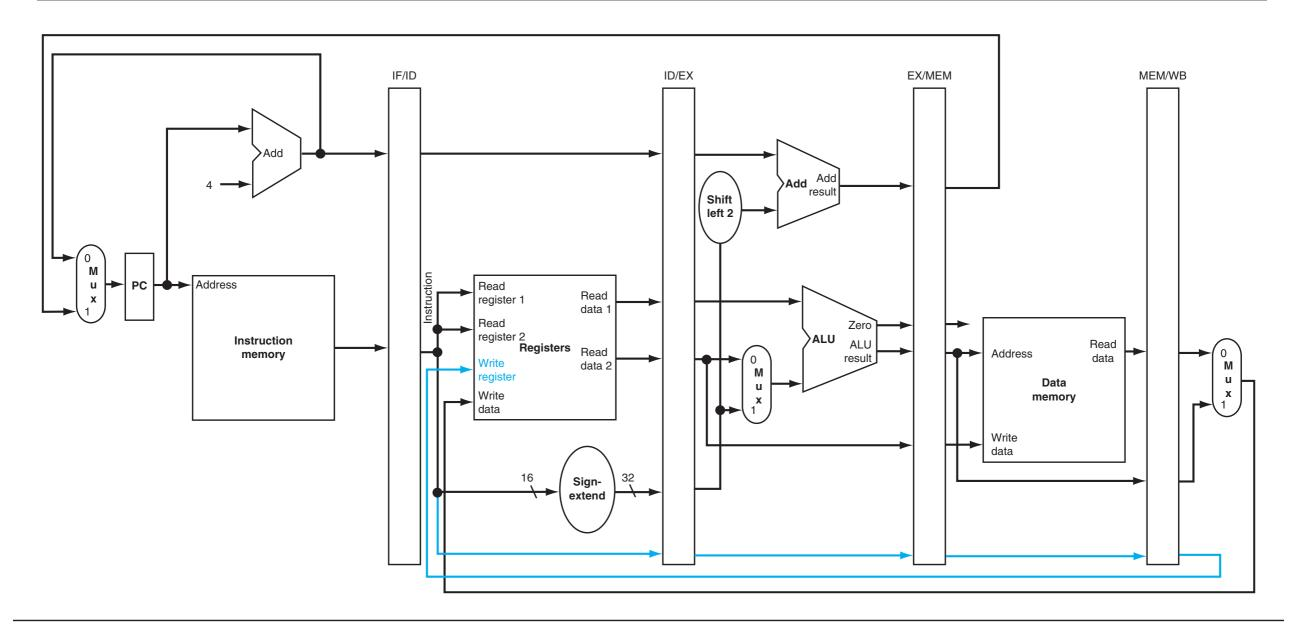
**FIGURE 4.41 The corrected pipelined datapath to handle the load instruction properly.** The write register number now comes from the MEM/WB pipeline register along with the data. The register number is passed from the ID pipe stage until it reaches the MEM/WB pipeline register, adding five more bits to the last three pipeline registers. This new path is shown in color. Copyright © 2009 Elsevier, Inc. All rights reserved.
