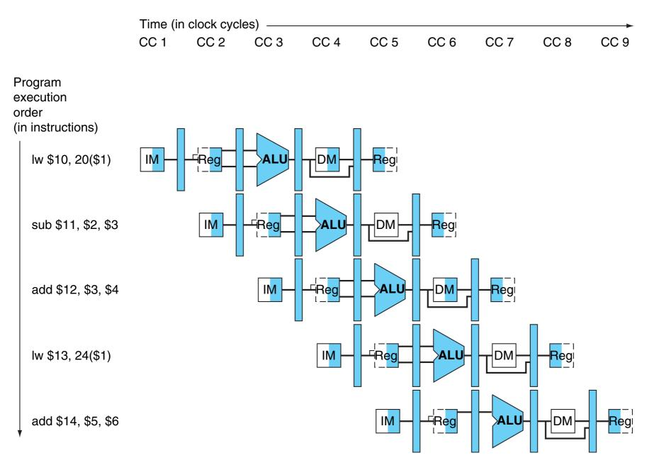
**FIGURE 4.43** Multiple-clock-cycle pipeline diagram of five instructions. This style of pipeline representation shows the complete execution of instructions in a single figure. Instructions are listed in instruction execution order from top to bottom, and clock cycles move from left to right. Unlike Figure 4.28, here we show the pipeline registers between each stage. Figure 4.44 shows the traditional way to draw this diagram. Copyright © 2009 Elsevier, Inc. All rights reserved.
