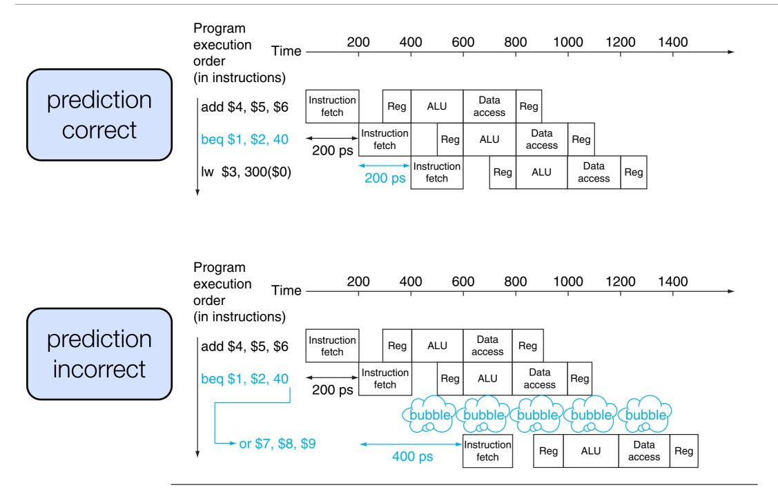
**FIGURE 4.32 Predicting that branches are not taken as a solution to control hazard.** The top drawing shows the pipeline when the branch is not taken. The bottom drawing shows the pipeline when the branch is taken. As we noted in Figure 4.31, the insertion of a bubble in this fashion simplifies what actually happens, at least during the first clock cycle immediately following the branch. Section 4.8 will reveal the details. Copyright © 2009 Elsevier, Inc. All rights reserved.
