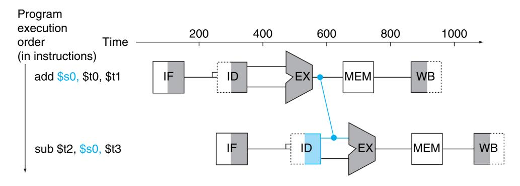
**FIGURE 4.29** Graphical representation of forwarding. The connection shows the forwarding path from the output of the EX stage of add to the input of the EX stage for sub, replacing the value from register \$s0 read in the second stage of sub. Copyright © 2009 Elsevier, Inc. All rights reserved.
