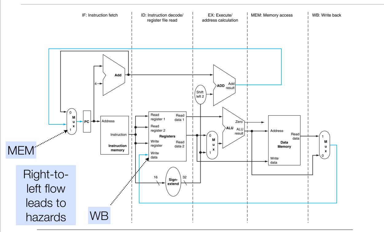
**FIGURE 4.33** The single-cycle datapath from Section 4.4 (similar to Figure 4.17). Each step of the instruction can be mapped onto the datapath from left to right. The only exceptions are the update of the PC and the write-back step, shown in color, which sends either the ALU result or the data from memory to the left to be written into the register file. (Normally we use color lines for control, but these are data lines.) Copyright © 2009 Elsevier, Inc. All rights reserved.
