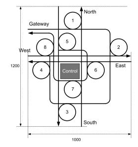
Fig. 5. Layout of photonic switch, showing waveguides and ring resonators. Units in microns.
