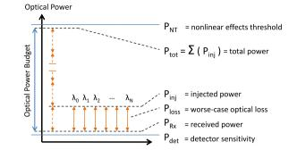
Fig. 8. Number of wavelengths dictated by insertion loss and optical power budget.
