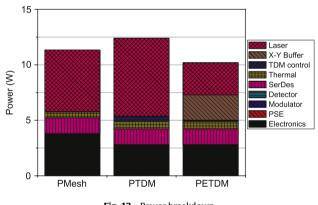
Fig. 12. Power breakdown.
