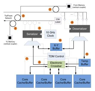
Fig. 6. Network gateway microarchitecture.
