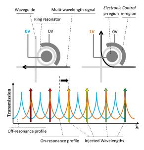
Fig. 1. PSE operation, switching from OFF to ON state, shifting wavelengths.
