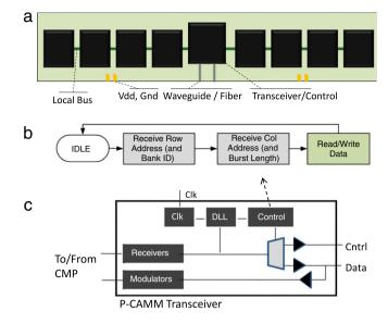
**Fig. 7.** Photonic Circuit-Accessed Memory Module design (a) Photonic CAMM (b) P-CAMM control logic (c) P-CAMM Transceiver.
