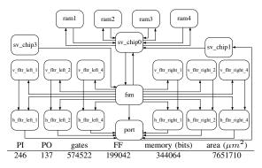
Fig. 3. The top-level block diagram of stereo\_vision based on its functional partition. Primary inputs and outputs are not shown.
