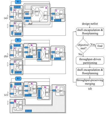
Fig. 1. (a) A simple LI system with four cores and one RS; its throughput is 2/3 = 0.67. (b) The same system with a finer-grained shell encapsulation where core *B* is split in two smaller cores  $B_1$  and  $B_2$ ; throughput is improved to 3/4 = 0.75. (c) The LI system maintains the same throughput after core *C* and *D* are merged. (d) The proposed high-level physical synthesis flow.
