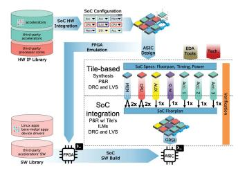
Figure 1: Proposed methodology for agile chip development.
