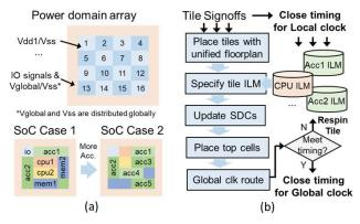
Figure 5: (a) Symmetric power domain array for flexible power cluster allocation, (b) Hierarchical timing closure flow.
