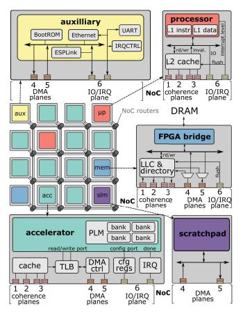
Figure 2: The ESP architecture and its five main types of tiles.
