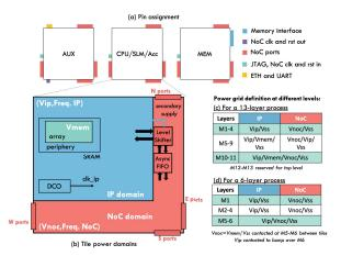
Figure 4: Breakdown of power domains and pin assignment.
