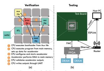
Figure 6: (a) Example of a full-system bare-metal simulation for verification, (b) The chip-testing environment.
